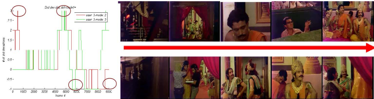
Fig. 6. Panels illustrate the story board generated for a viewing session over the clip jbdy . The PD information is smoothed using a moving average and large deviations from the mean are isolated. Local maxima and minima are then identified as shown in the inset to the left. The key frames sampled from this process are shown in sequence (left to right, top row then second row). The frames were rated by the user to contain 6 of 10 key events. Frames are from the video jbdy , copyright owned by the National Film Development Center, India.
